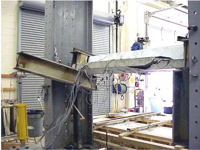
**Figure 3.** Strengthened Specimen (TB2) Failure Mode
