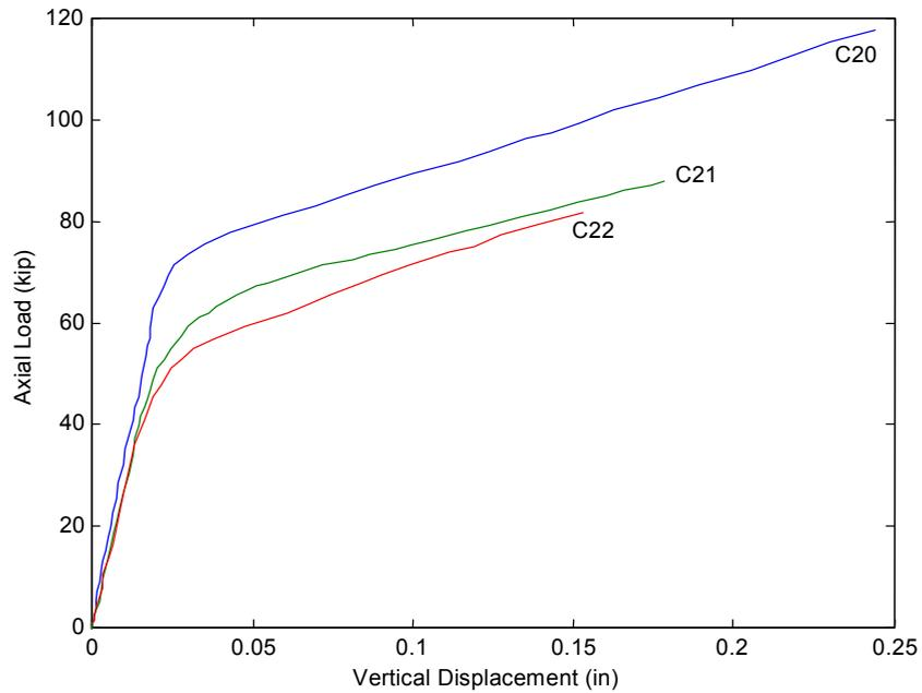
**Figure 5.** Load-Deflection Curves for Specimens with Two Layers of FRP Jacket
