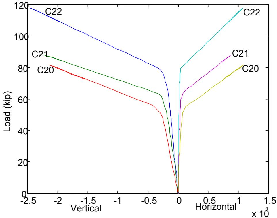
**Figure 6.** Vertical and Horizontal Strains at Mid-height for Specimens with Two Layers of FRP Jacket
