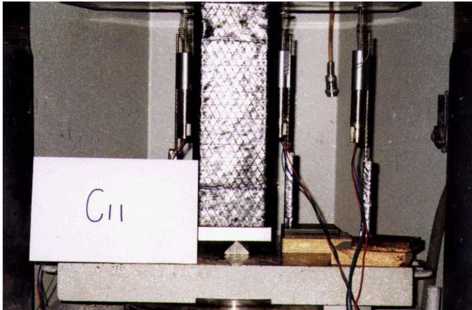
**Figure 1.** Test Setup for Columns with Eccentric Loadings
