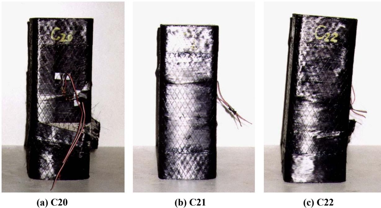
**Figure 2.** Specimens with Two Layers of FRP after Failure
