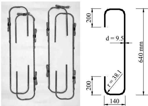
Figure 2. Details of the used carbon FRP stirrups
