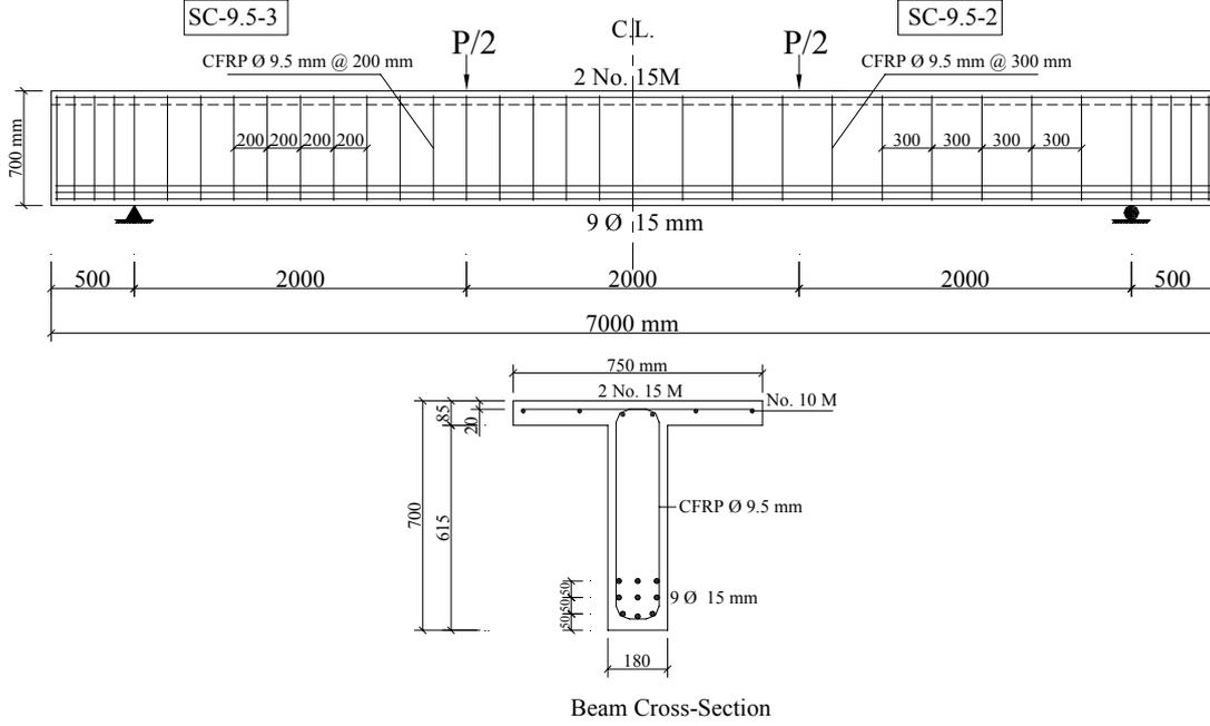
Figure 1. Geometry and reinforcement details of test beams.
