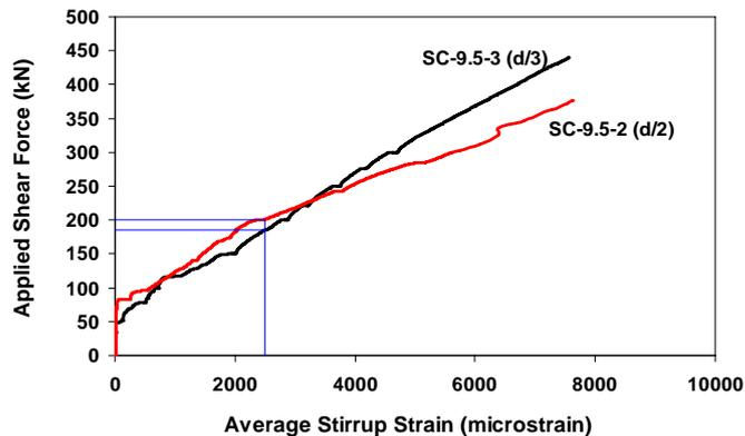
Figure 6. Applied shear force-average stirrup strain relationship.
