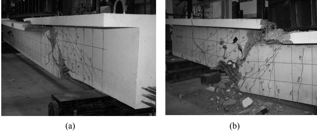
Figure 4. Shear failure of test specimens: a) SC-9.5-2 (d/2); b) SC-9.5-3 (d/3).
