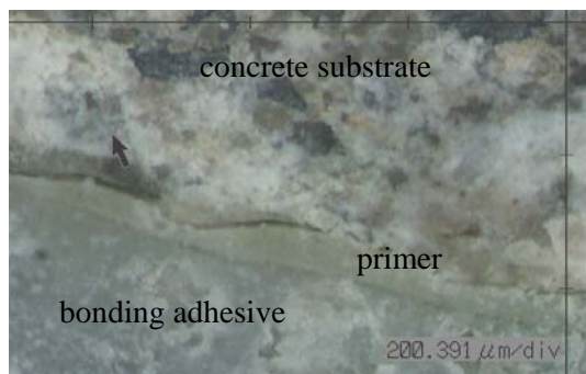
Figure 4. Microscopic observation on the interface bond
