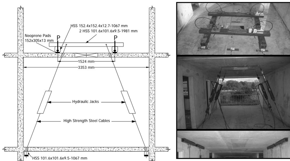
Figure 3. Cross-sectional elevation of the test setup.
