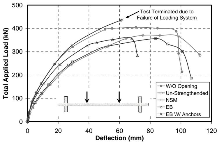
Figure 7. Load-deflection envelopes of test slabs.
