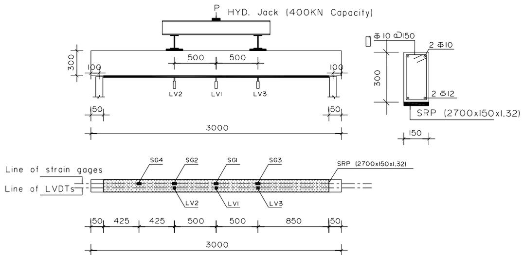
Figure 3b. Test setup
