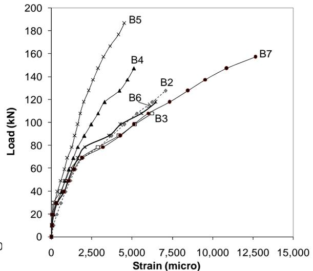
Figure 7. Load-tensile strain behavior
