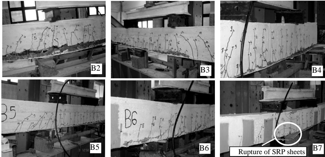
Figure 8. Failure modes of different specimens
