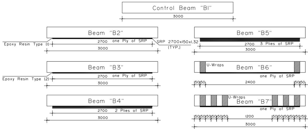
Figure 3a. Details of the test specimens
